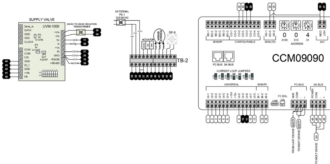
FIGURE 35: CCM EXHAUST VALVE SYSTEM
