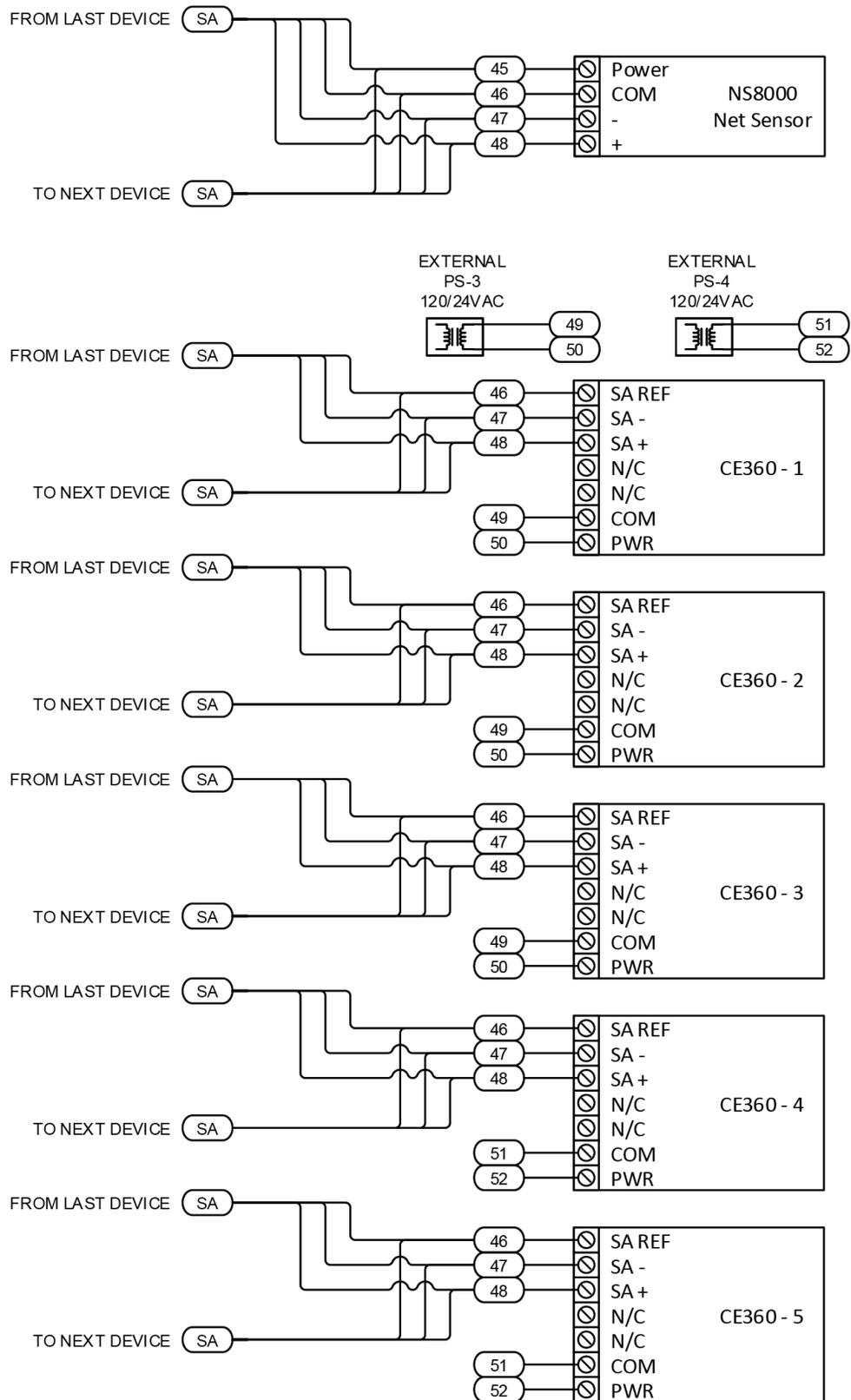
FIGURE 37: CCM UVM SUMMING WIRING
