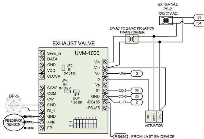
FIGURE 36: CCM TERMINAL BLOCK
