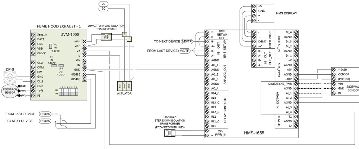
FIGURE 31: FMS DISPLAY SYSTEM WIRING
