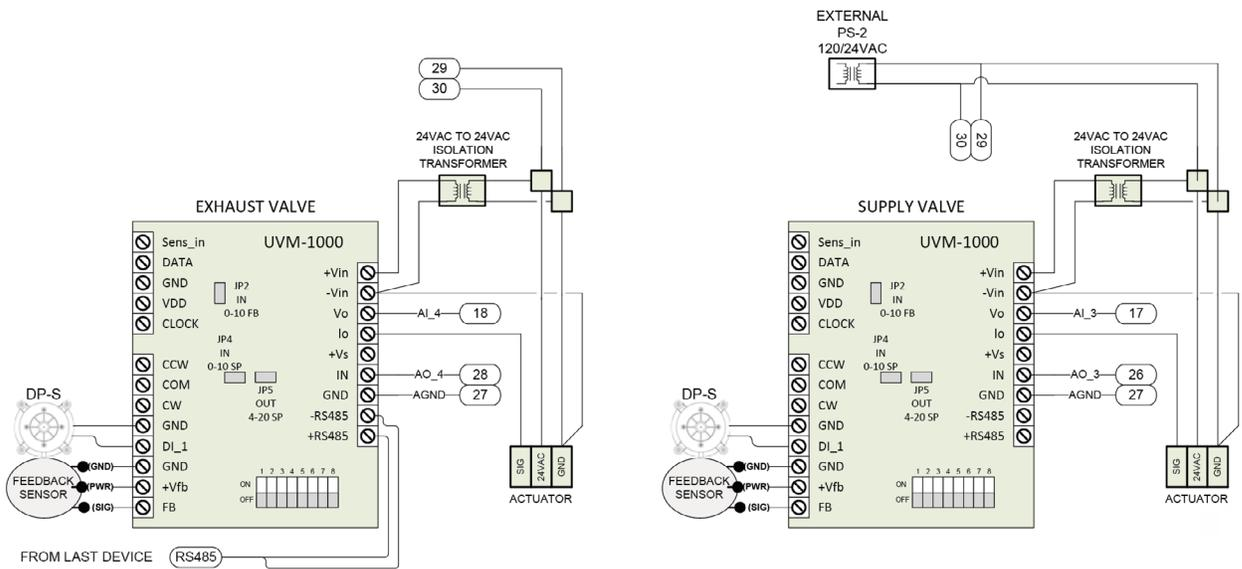
FIGURE 30: FUME HOOD EXHAUST TO HMS DISPLAY SYSTEM WIRING
