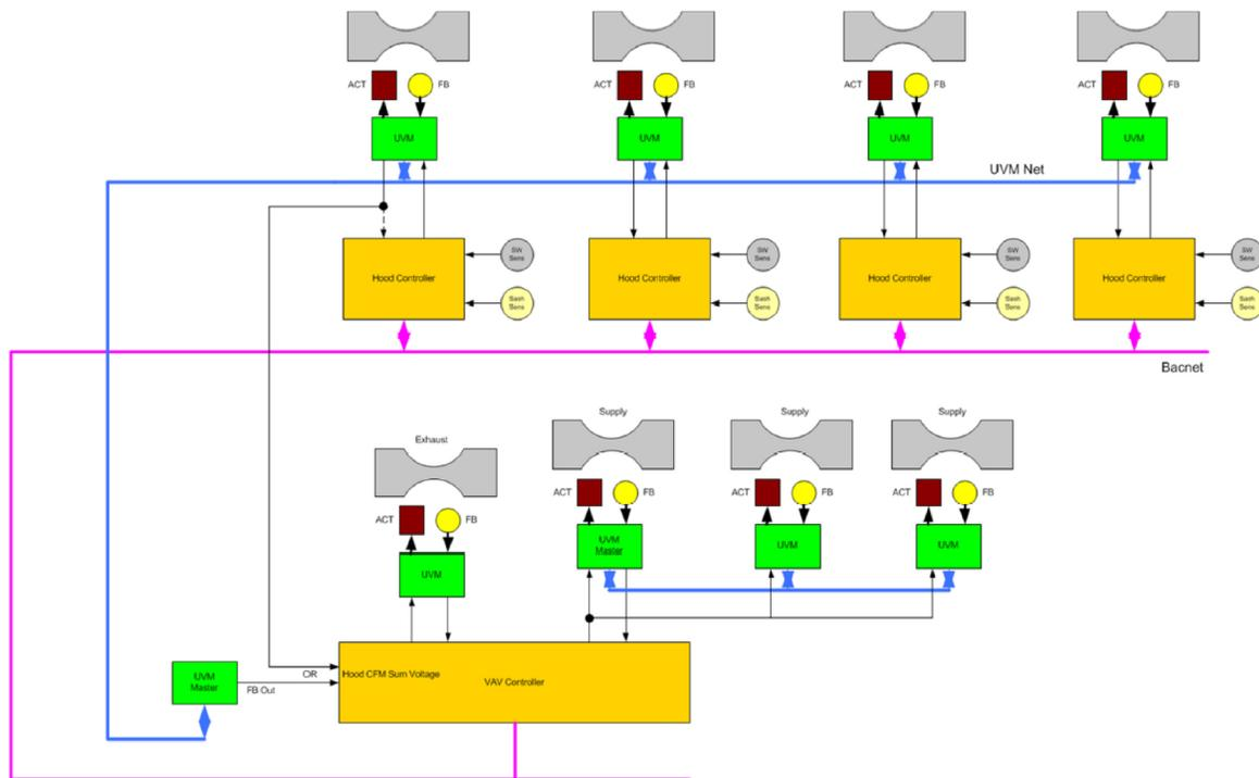
FIGURE 25: UVM SUMMING WIRING DIAGRAM
