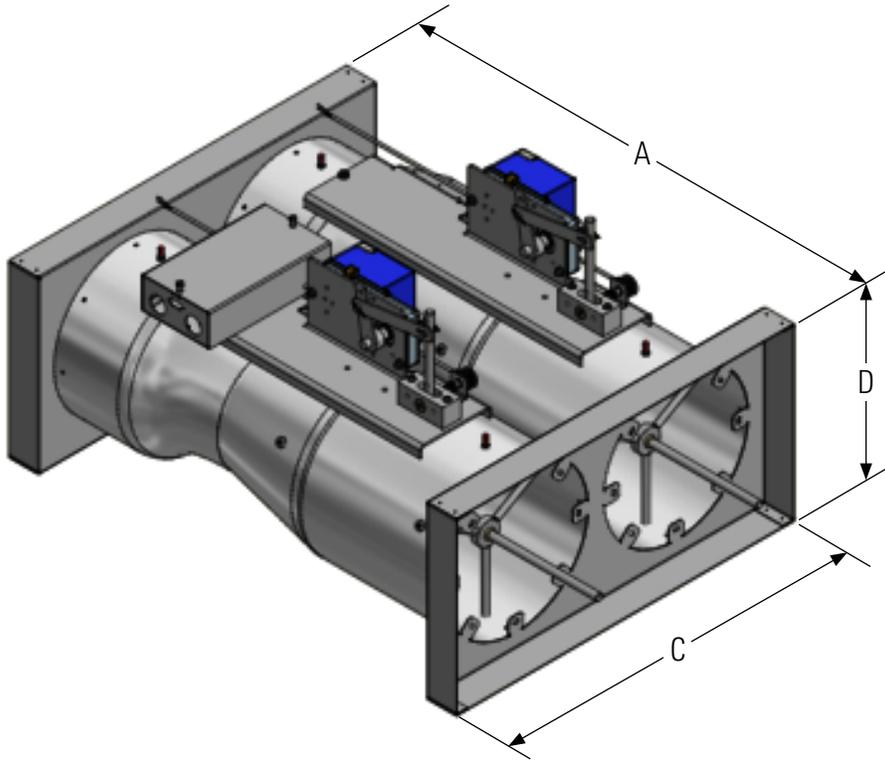
FIGURE 8: TRIPLE VENTURI VALVE
