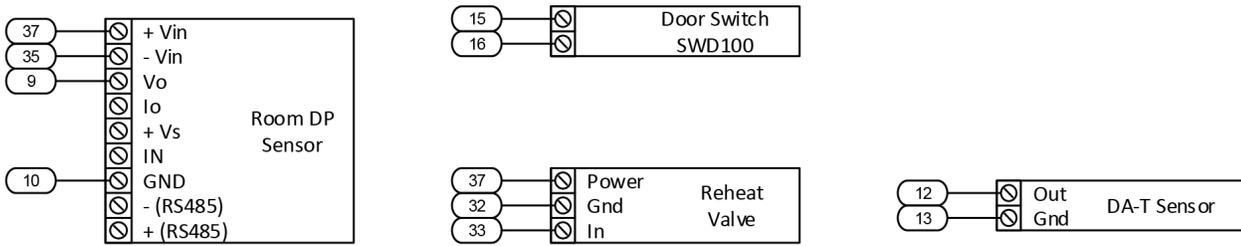
FIGURE 38: FUME HOOD EXHAUST TO HMS DISPLAY SYSTEM WIRING
