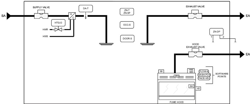
FIGURE 34: CCM SUPPLY VALVE AND CONTROLLER SYSTEM
